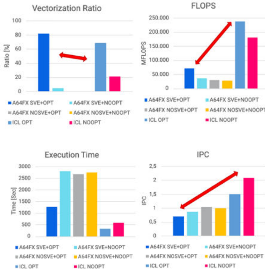
FIGURE 26: HISTOGRAM OF THE METRIC FOR SPCFEM3D SIMULATION ON IRENE (A64FX) AND GALILEO100 (ICL) WITH OR WITHOUT SVE AND CHEESE OPTIMIZATIONS.
