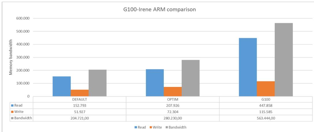
Figure 27: Comparison between OPT and DEFAULT version for HBM metric on Irene@TGCC and Galileo100@CINECA)
